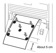
**10**Remove the paper from the front side of the cleaning sheet.
